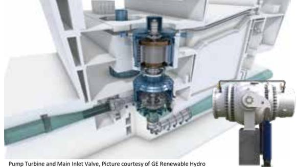
Pump Turbine and Main Inlet Valve, Picture courtesy of GE Renewable Hydro
